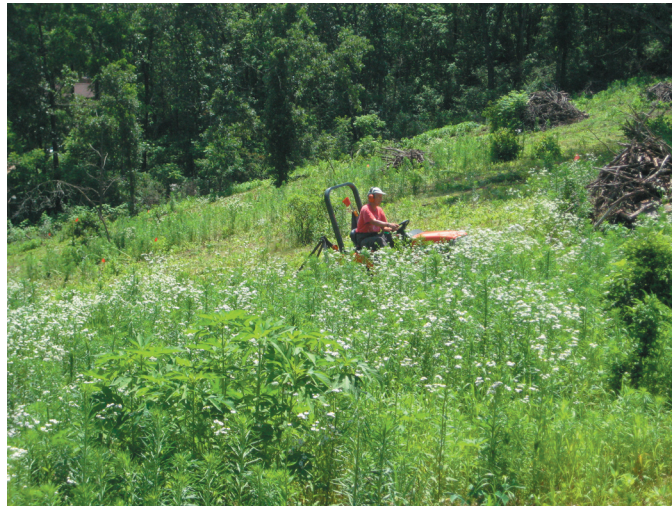
Mowing the East Basin in mid summer. The Kubota tractor pulling a small bush hog worked fairly well for this task. Obstacles such as big rocks or large stumps that had not been cut low enough were marked with flags and cut around. Because of the steepness of the hill, mowing had to be done in a vertical direction. Even with great precautions, there were still some dangers involved. Kathie did all the mowing. Top, Figure 40. June 16, 2010. (IMG_6971.jpg) Middle, Figure 39. June 20, 2010. (IMG_7005.jpg) Bottom, Figure 41. June 22, 2010 (IMG_7030.jpg)
